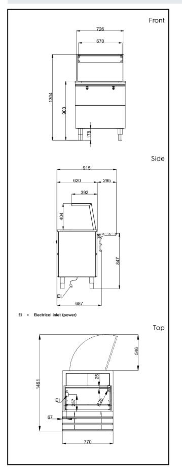
Flexy Compact Tempered glass top on cupboard (2GN) with overshelf with LED lights, H=900mm The company reserves the right to make modifications to the products without prior notice. All information correct at time of printing.
